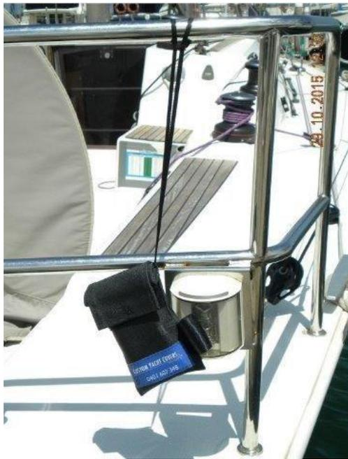
2. Wrap the Velcro straps around horizontal and vertical rails as shown below.
