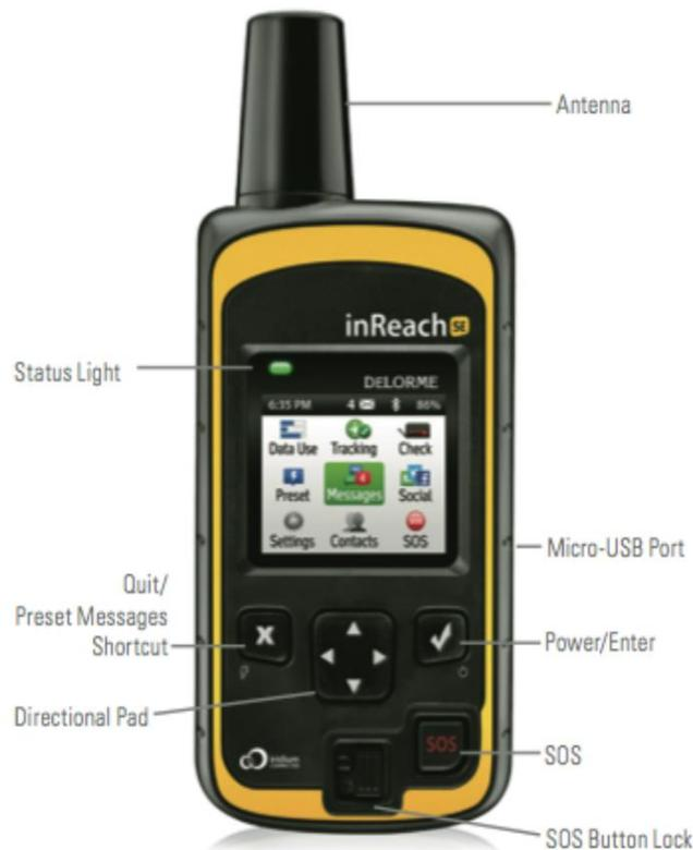
**Antenna** - Keep the satellite communicator antenna pointing up, with a clear view of the sky and not obstructed by parts of your boat.
